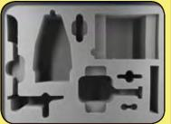
Using our CNC router we can custom cut specialised foams to fit your equipment. Two types of foam are available, Anti-shock Polyethylene or Flame Retardant Anti Static foam (FRAS)
