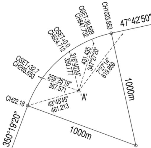
Using the diagram as shown on the left for this example you will compute setout bearings and distances by entering the known chainage and offset.
