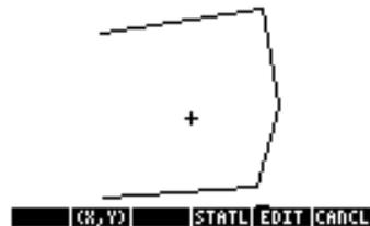
Hitting the menu key **B** labelled **(X,Y)** displays the coordinates system within the entered close ( Start is 0,0 ). The cursor can then be moved around the screen. Initiate menu key **F** labelled **CANCL** or the **ON** button to exit to the previous menu.
