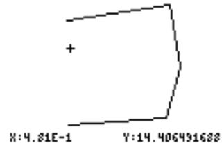
Note: The plot does not display the arc information of the entered curve data, however a straight line is plotted in its place from the end points of the arc.
