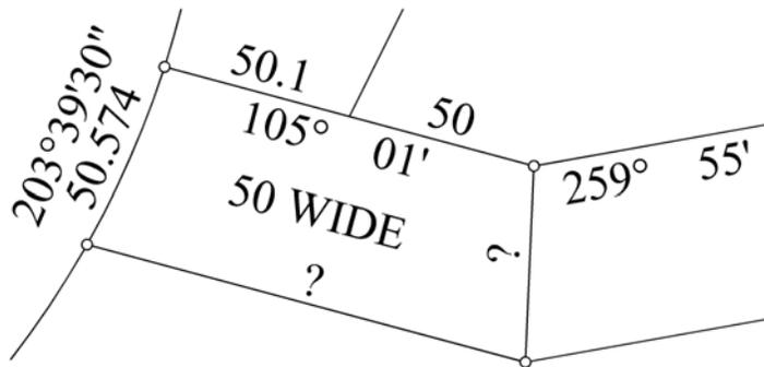
As can be seen in this example there is not enough information to solve the unknowns straight away without first working out the 1/2 angle solution.
