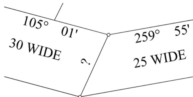
The Secant routine computes the join between two sets of parallel lines with two different offset distances.
